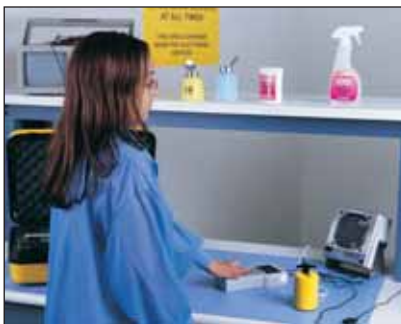
Figure 6: ESD mat with test kit
