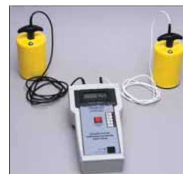
Figure 5: Surface resistance meter
